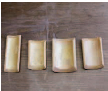
Bamboo scrapers are for smoothing the round sides of pot bodies.
