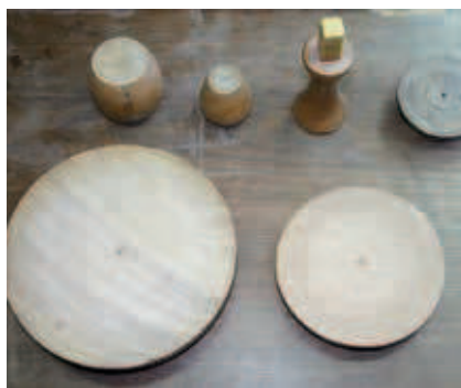
Wheels for spinning the pot and round blocks for a smooth mouth.
