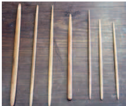
Bamboo picks for cleaning, opening and smoothing small holes.
