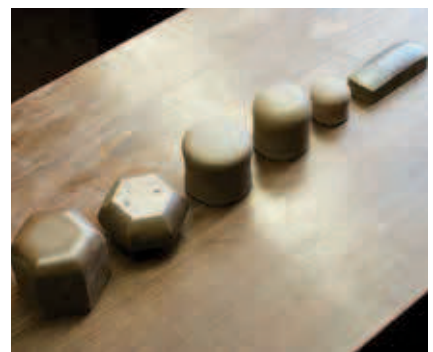
Various tools for smoothing the inside of the mouth, depending on shape.
