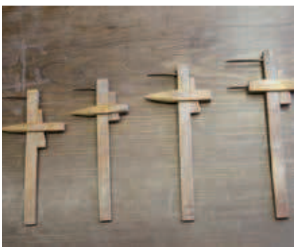
Calipers are for cutting circles or measuring clay to fit together.
