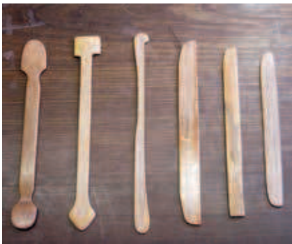
These bamboo tools are for shaping and decorating details of the pot.
