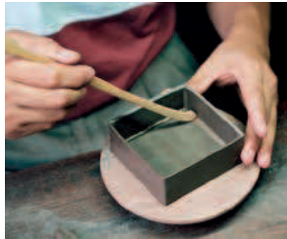
The creases of the joints are then smoothed out and refined.
