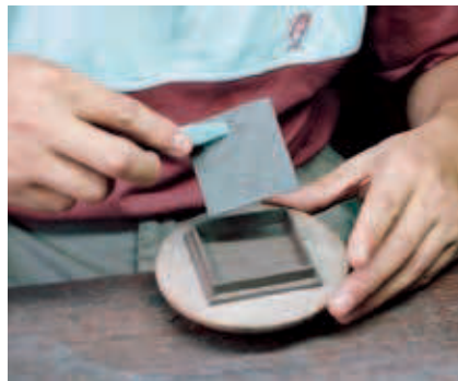
The lid and button are joined together and refined until they are smooth.
