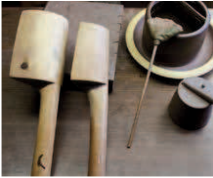
Mallets for flattening clay into strips to form the body.
