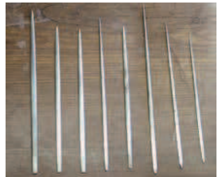
Metal picks for even finer details and for making sieve holes.
