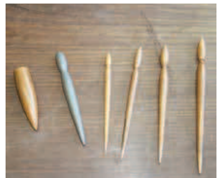
These round pegs are for smoothing the spout and button holes.
