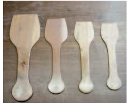
Paddles are for shaping the body of pots by slapping the sides.
