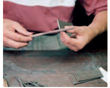
Wet slip is applied to the sides of each of the pieces.
