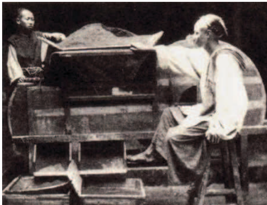
茶 Very early photograph of a winnowing machine used to separate the leaves. The stalks and little bits were separated by the spinning machine, saving the workers a lot of time, since sorting the leaves by hand on trays is very inefficient and time-consuming. Of course, the tumbling of the leaves would also damage some, however, resulting in a lower-quality tea.
